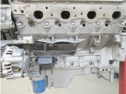
Passenger Side - to be fitted as per picture, using the front 4 mounting holes on the engine block. The Passenger-side Engine mount bracket is marker I 69
