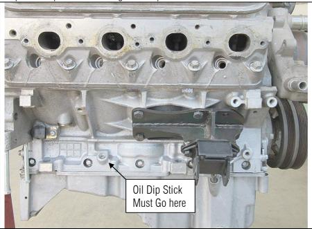
Drivers Side - to be fitted as per picture using the front 4 mounting holes on the engine block. The Driver-side Engine mount bracket is marker R69.
